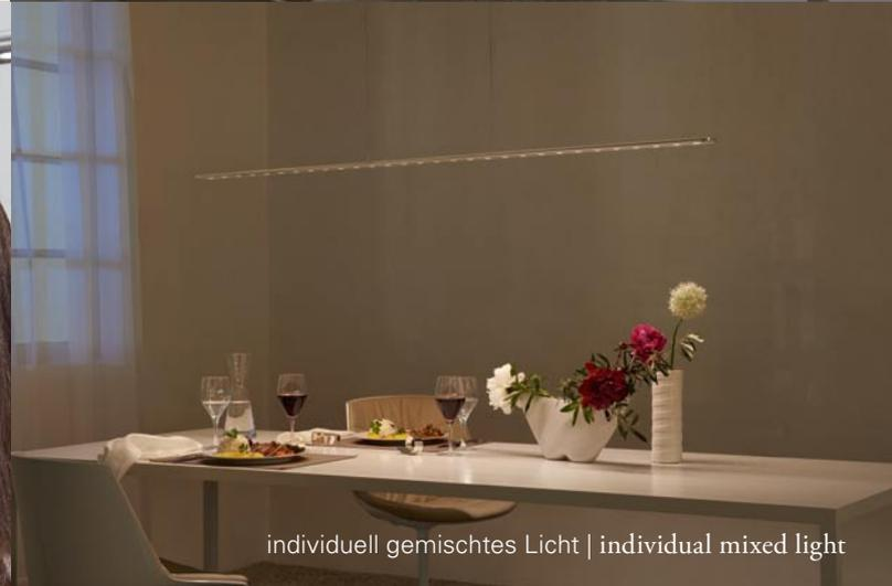
You only need to briefly touch the capacity sensor at the bottom surface of the pendant lamp to switch the light colour one step further. Different white tones of 2700 Kelvin (warm white) to 5700 Kelvin (cold white) can be adjusted. A longer touch dims the brightness level. When the light is switched off, the selected light colour and brightness level are stored.
